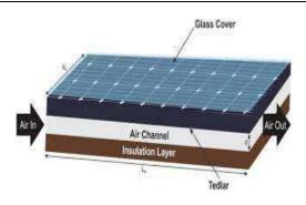
Figure 3: Glass installed on collector frame
